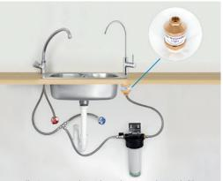
Installation example with Carbonit under-sink filter.
